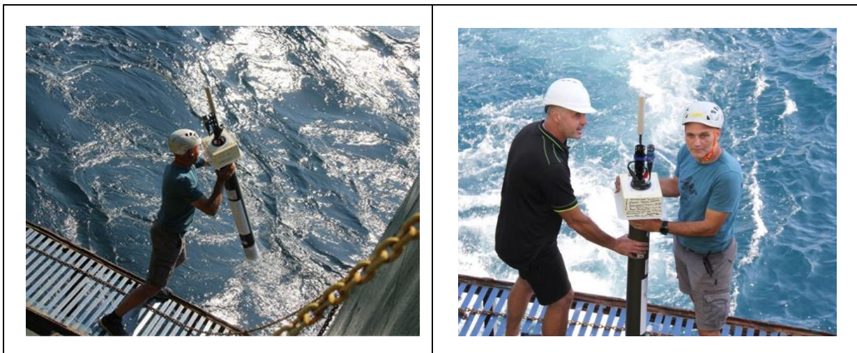
Figure 2. Deployments of Bulgarian Argo floats from R/V Mare Nigrum as part of the STREAM-DANUBE cruise. ©IO-BAS
